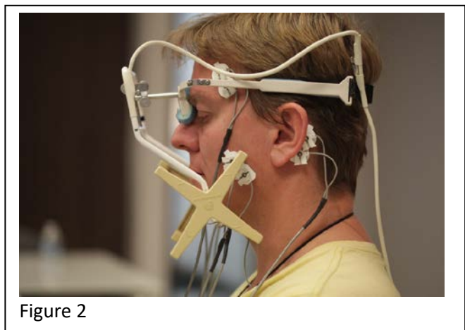
Figure 2 Figure 2: K7 Kinesograph: Computerized mandibular scanning (CMS – jaw tracking) and electromyography (EMG) (Myotronics-Noromed, Inc, Kent, WA) is used to measure and monitor jaw positioning and muscle activity objectively.
